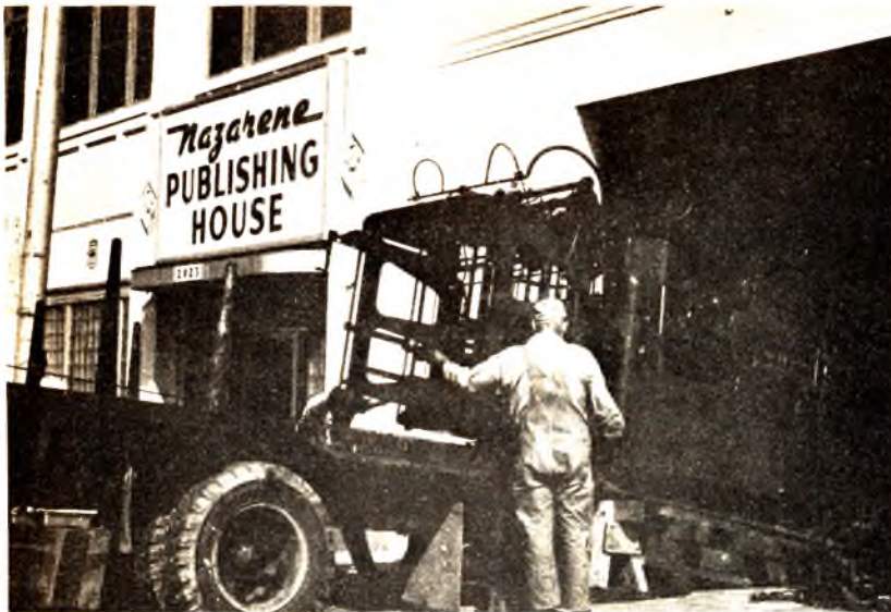
OUT COMES THE OLD —A Miller letterpress, long a tool of the printers at the Nazarene Publishing House, disappears from the scene as the production department continues to modernize with the increased use of lithography. While the old press was being removed, a new lithographic press was being installed in the offset division across the street from the letterpress section.
